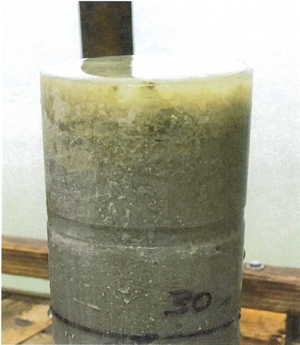
Figure 2. Sediment core taken immediately after the May 2017 alum treatment in middle Pelican Horn. Alum floc shown at the surface.
