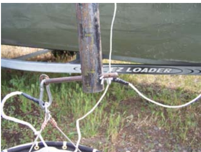
Figure 8. Cotter pin of quick release system used to sample larval fishes on Moses Lake, Washington.
