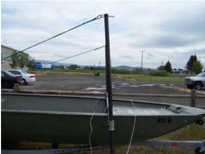
Figure 7. Straight post of quick release system used to sample larval fishes on Moses Lake, Washington.
